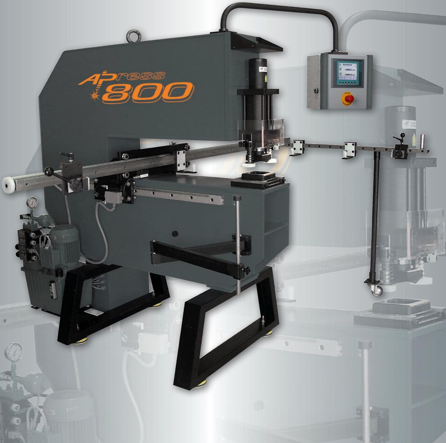
The stationary hole punch has been developed for control cabinet and switch gear makers and is suitable for quick punching-out of circular, square, rectangular or special forms in sheet metal and control cabinet doors up to 2200 mm x 1000 mm and 40 mm margin fold height. Punching possible right up to margins. Simple, rapid tool change carried out in seconds - even on fitted door. Limit stop system can be moved in X and Y directions.
