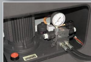
Dual-circuit hydraulic unit in cabinet base
