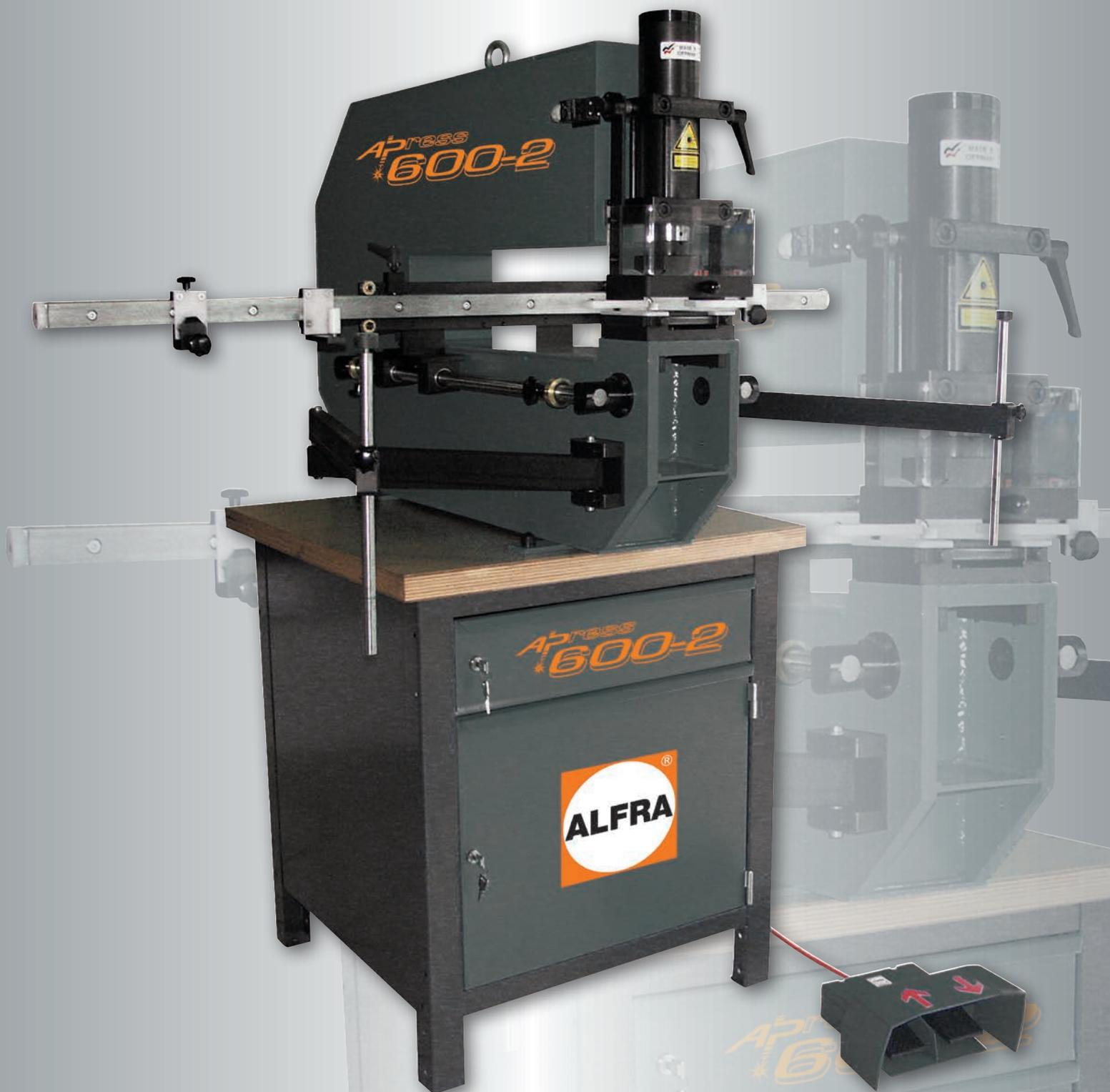
The stationary hole punch has been developed for control cabinet and switch gear makers and is suitable for quick punching-out of circular, square, rectangular or special forms in sheet metal and control cabinet doors up to 2200 mm x 1000 mm and 30 mm margin fold height. Punching possible right up to margins. Simple, rapid tool change carried out in seconds - even on fitted door. Limit stop system can be moved in X and Y directions.
