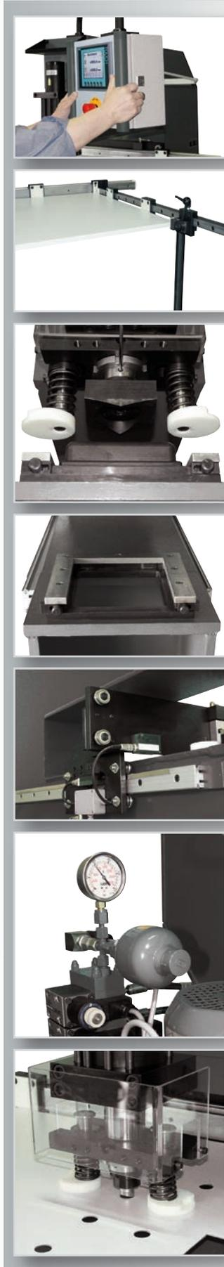
*Pivoting control panel with two-hand operation*
