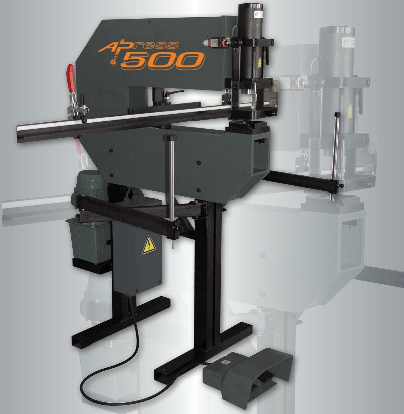
The stationary hole punch has been developed for control cabinet and switch gear makers and is suitable for quick punching-out of circular, square, rectangular or special forms in sheet metal and control cabinet doors up to 2000 mm x 1000 mm and 30 mm margin fold height. Punching possible right up to margins. Simple, rapid tool change carried out in seconds.
