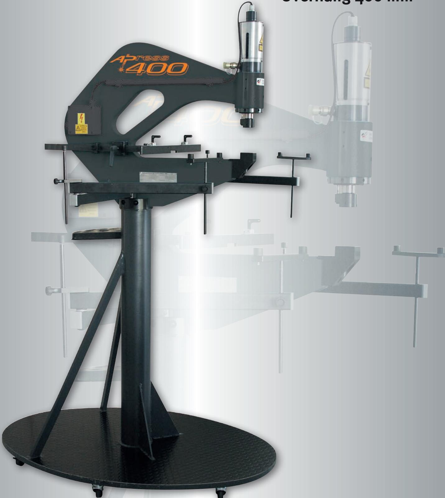
For rapid punching-out in circular, square, rectangular or special forms without pre-drilling in control cabinet doors, terminal boxes, cable ducts, housings, cable management panels etc. right up to margins. Simple tool change carried out in seconds.
